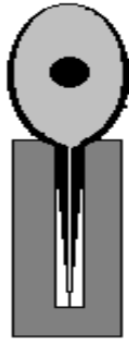
FIG.2: Epoxy fiberglass forms a mold to hold the two edges of the NbTi foil together. The NbTi wire is inserted inside the cylinder of NbTi foil
