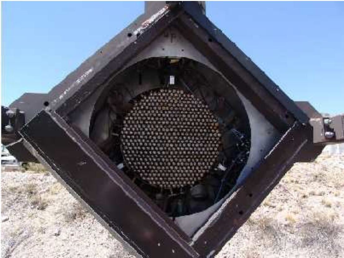
Fig. 2.— Telescope Camera Box, located at the focus of the telescope reflector. In the center is a high resolution, 499 PMT camera. Taken from Holder et al. (2006).
