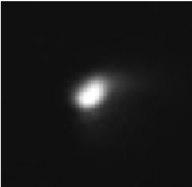
FIG. 3: This is a typical picture of the focal spot. It is slightly deformed, since the laser is operating at the lowest possible power. Each pixel is 5.6\mu\text{m} in width and height.
