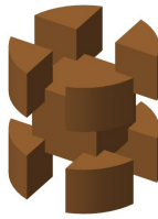
FIGURE 4. \vec{B} core. Each axis is wound around the center cube, and the eight feet keep the coils in place.
