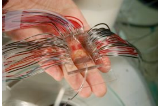
Figure 3: Microfluidic device developed at UCLA capable of running 1,000 chemical reactions simultaneously.
