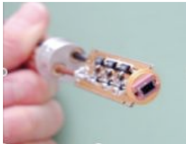
Figure 12: Small electron detector, which could potentially plug into lab-on-a-chip SEM.
